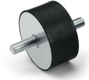
Fig 10. Rubber vibration isolators (e.g. Ø60: DVA.1-60-40-M10-28-40) in accordance with the manufacturer's standards in terms of weight and size of the unit, providing support over the full width of the unit foot.
