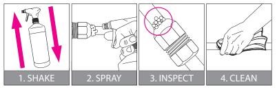
Spray onto suspect joints to achieve an even coating. Large leaks bubble up immediately; slow, small leaks bubble up within a few seconds or minutes. When leak detection has been completed, wipe inspected areas with a damp cloth.
