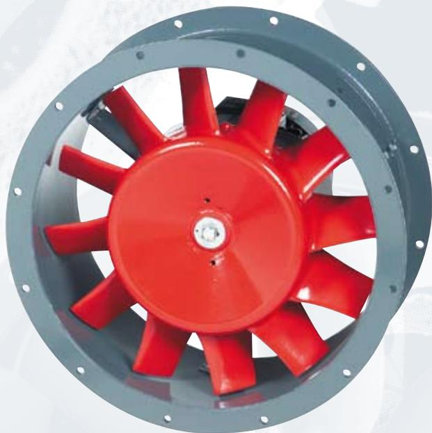
Range of axial flow fans fitted with two pole motors for high pressure applications. Casings are formed from rolled steel sheet finished with grey epoxy-polyester paint coating. All models incorporate one piece die-cast aluminium impellers. The impellers are finished in a red colour epoxy-polyester paint coating.
