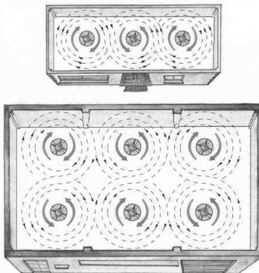
The choice the first unit's rotation is not important as long as the following units are installed with alternate rotations; it is not important what rotation the last unit has.
