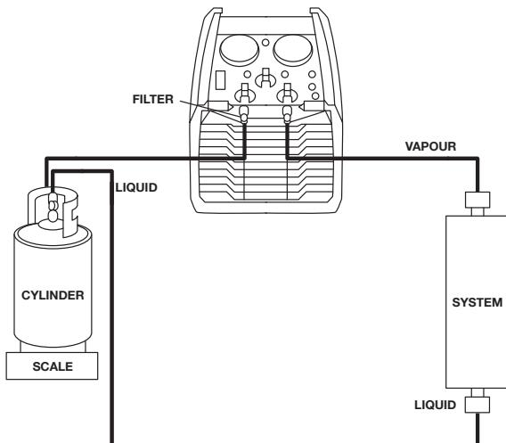
4.4.1 The PUSH PULL method is used to move a large amount of liquid refrigerant from the system being serviced to the recovery cylinder without passing it through the compressor. This method is only useful when more than 7 Kg of liquid is known to be in the system and it can be easily isolated. DO NOT ATTEMPT the PUSH PULL process unless you are sure of the situation.
